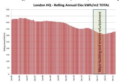
building to achieve a substantial 17% reduction in its overall consumption with 60% of this likely to be due to improvements in HVAC system control and equipment. The consumption also showed an improvement, which corroborates the improvements seen in ventilation rate control as this affects the amount of heating needed of the incoming air.
