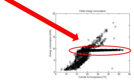
These electricity savings represent a reduction of 33 % from the initial electricity energy use on HVAC system.
