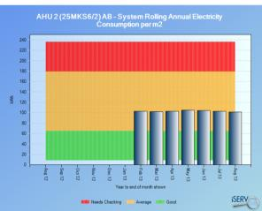
Impact on lower electricity energy consumption has a cold storage system (the results are shown in pictures above) which is already installed on building. Cold storage is also useful for shifting some of peak load, particularly cooling requirement, to the late evening and early hours in the morning. It was found that cold generator load shifting using thermal cold store could reduce the peak building load by 15%.
