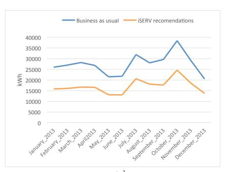
reduction of the HVAC annual building energy use can be reduced to 40.5 kWh/m<sup>2</sup>.year. It is not possible to know the total building savings, because there is no meter in the main electricity board.
